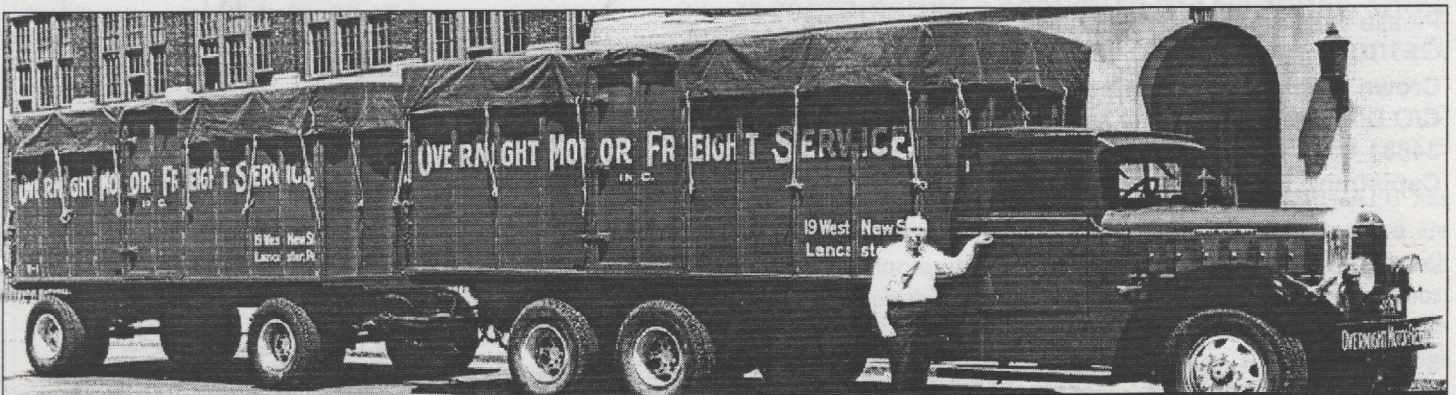
1934 GMC T-96 Six-Wheeler truck with GMC trailer. Photo from Pictorial History of American Trucks by Niels Jansen, Elmar Published 1994 in association with Bay View Books Ltd.
