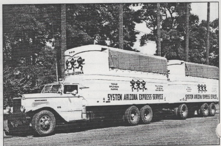
1937 Autocar Diesel Model NF 6x2 truck and trailer. Photo from Pictorial History of American Trucks by Niels Jansen, Elmar Published 1994 in association with Bay View Books Ltd.
